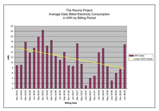
This graph brings grid usage down to the daily level. The fall off in daily grid usage is dramatic especially in the summer time, the peak generation time of the year.
