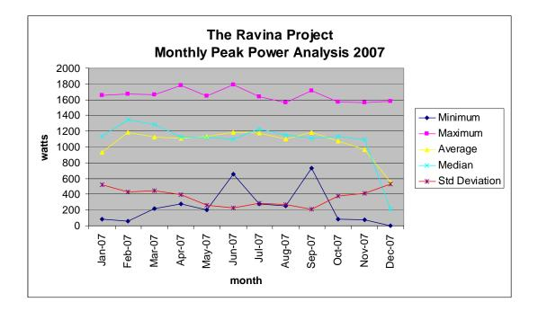
The graph above is set up to show the value of the maximum and minimum peak power recorded for each month. During poor months the minimum peak power might only be 100 watts or less, even zero. These are very poor days with the sky in dull overcast all day long.  $\otimes$
