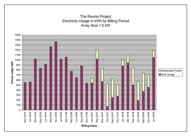
Using our old utility bills and combining them with our daily readings for energy generation we can produce a graph showing exactly the effect our solar array is having upon the demands the house is making upon the electrical grid.
