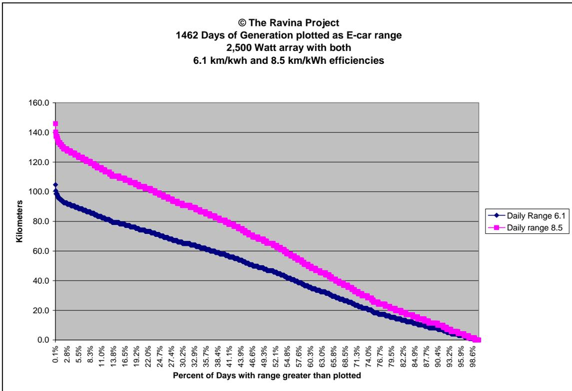
We assume we have upgraded our array to 2,500 Watts, generated 4 years of data and calculated the range we could drive the next day based upon the amount we generate on any given day. On day 1 we generate 'x' amount of energy. On day 2 we translate this energy into our driving range budget for that day. The results are placed upon the graphic above for the two efficiency ranges, 6.1 and 8.5 km/kWh.
