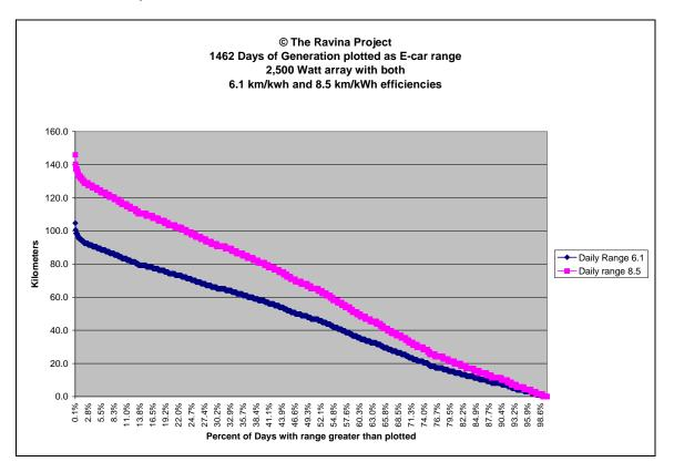
We assume we have upgraded our array to 2,500 Watts, generated 4 years of data and calculated the range we could drive the next day based upon the amount we generate on any given day. On day 1 we generate 'x' amount of energy. On day 2 we translate this energy into our driving range budget for that day. The results are placed upon the graphic above for the two efficiency ranges, 6.1 and 8.5 km/kWh.
